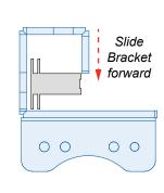
Tighten thumb screws to secure connection to inside of frame.
