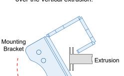
2 Slide bracket forward, then down onto V4 connector.
